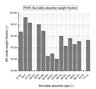
FIGURE 5. PWR burnable absorber weight fraction.
