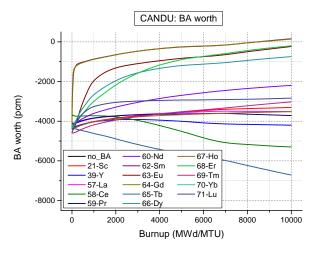
FIGURE 10. CANDU burnable absorber worth during fuel depletion.
