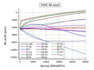
FIGURE 11. PWR burnable absorber worth during fuel depletion.
