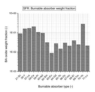
FIGURE 6. SFR burnable absorber weight fraction.
