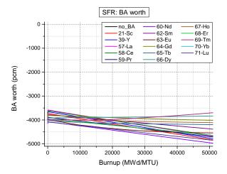
FIGURE 12. SFR burnable absorber worth during fuel depletion.
