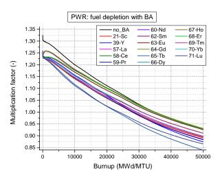
FIGURE 8. PWR multiplication factor during fuel depletion.
