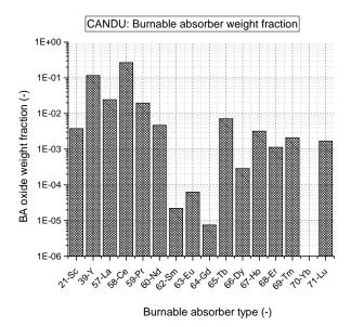
FIGURE 4. CANDU burnable absorber weight fraction.
