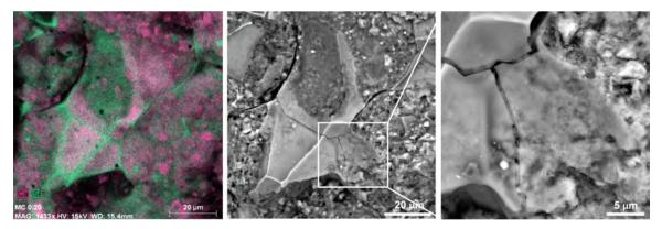
FIGURE 3. SEM – EDS of integrated perlite fines – Si content decrease and detail of lamella integration.
