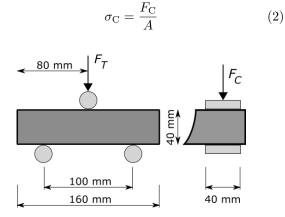
FIGURE 1. Macroscopic tests setting – three-point bending (left), compression (right).
