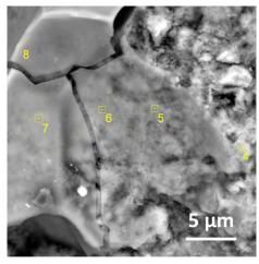
FIGURE 5. EPMA – EDX of perlite lamella and cement.
