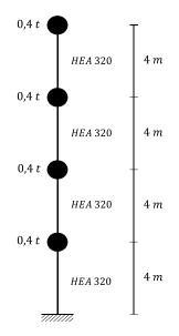
FIGURE 1. Structure of the 4-dof system.
