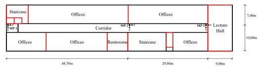
FIGURE 4. Floor plan of the story 6 of the RC-building.
