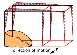
FIGURE 6.  $2^{nd}$  modal shapes of 7-story RC-building identified by using FDD.
