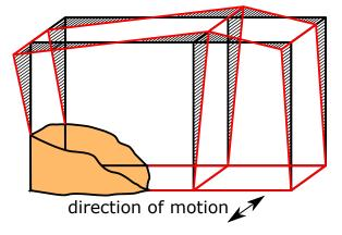
FIGURE 7.  $3^{rd}$  modal shapes of 7-story RC-building identified by using FDD.
