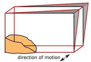
FIGURE 5.  $1^{st}$  modal shapes of 7-story RC-building identified by using FDD.
