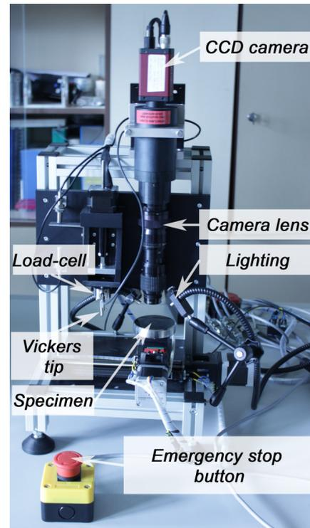
FIGURE 2. Experimental setup.
