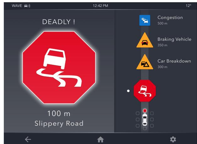
FIGURE 2. Three-stage warning GUI.
