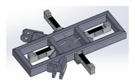
FIGURE 3. Load sensors attachment.
