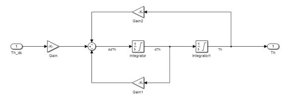
Figure 5. Mathematical model of the direct dynamic response – rubber ball.
