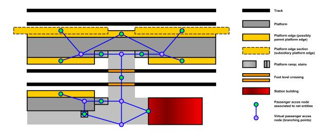
FIGURE 3. An author's proposal of RailTopoModel application in the scope of passenger routing issue exemplified for the case of a railway station equipped with platforms with level access.
