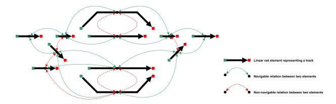
FIGURE 1. An application of the RailTopoModel principles on an example of a railway station with five simple turnouts and one single slip modelled by the means of positioned net relations.
