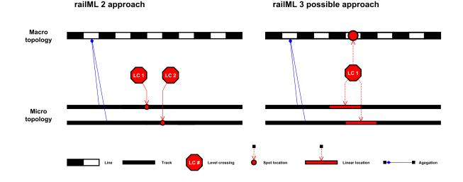
FIGURE 2. Illustration of different approaches in locating of entities in the scope of railML 2 and railML 3.
