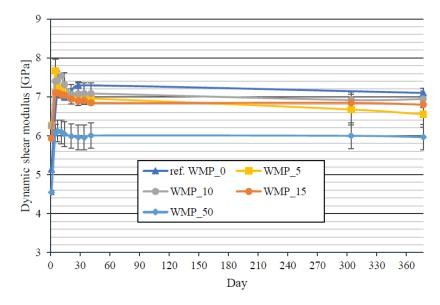
FIGURE 3. Time dependence of dynamic shear modulus (with standard deviation).
