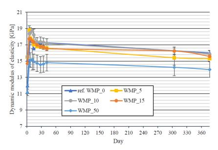
FIGURE 4. Time dependence of dynamic modulus of elasticity (with standard deviation).
