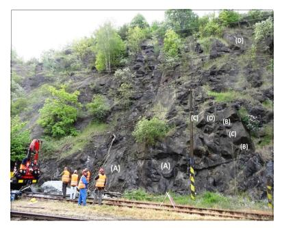
FIGURE 2. Discontinuity systems on the rock wall being monitored.
