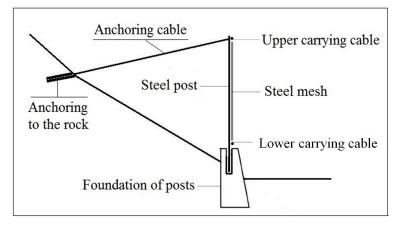
FIGURE 8. Protective fence – schematic cross section.
