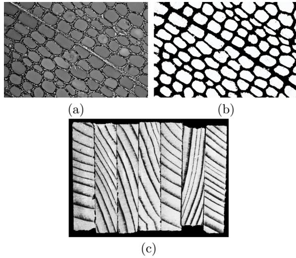
FIGURE 2. a) Original gray-scale image of earlywood, b) Transformed binary image of earlywood, c) Images of growth rings.
