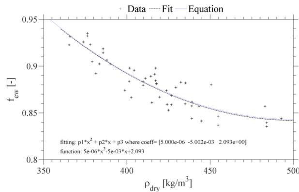
FIGURE 3. Dependence of the earlywood volume fraction on dry wood density [kg/m<sup>3</sup>].
