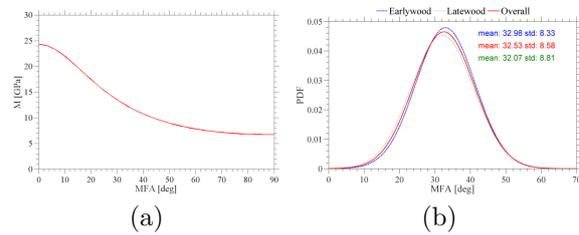
FIGURE 1. a) Variation of indentation modulus as a function of MFA, b) Probability density function of MFA
