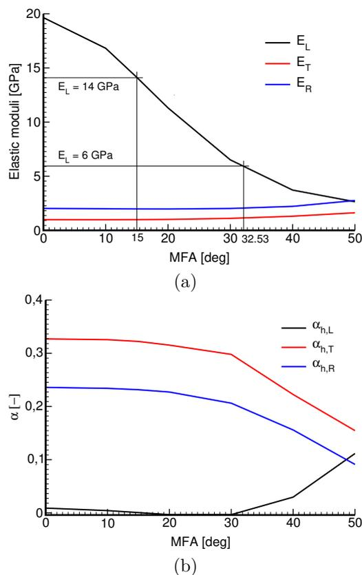
FIGURE 6. Variation of selected homogenized properties as a function of MFA: a) elastic moduli, b) coefficients of hygroexpansion.
