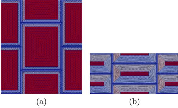
FIGURE 5. Geometry and plane view of discretized PUCs: a) earlywood, b) latewood.
