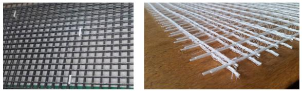
FIGURE 2. 2D carbon and 3D glass textiles.
