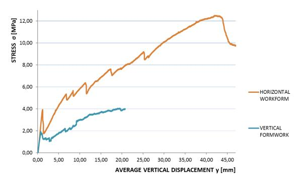
FIGURE 7. The flexural testing of TRLC slabs with 3D glass textile.
