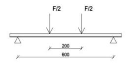
FIGURE 5. The static scheme of slab loading.
