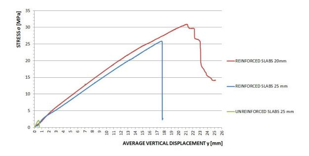
FIGURE 6. The flexural testing of TRLC slabs with 2D carbon textile.
