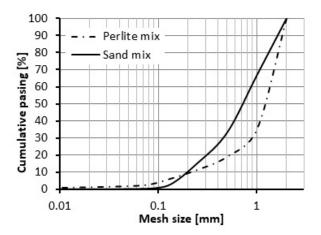
FIGURE 1. Sieve analysis of perlite and sand mix.
