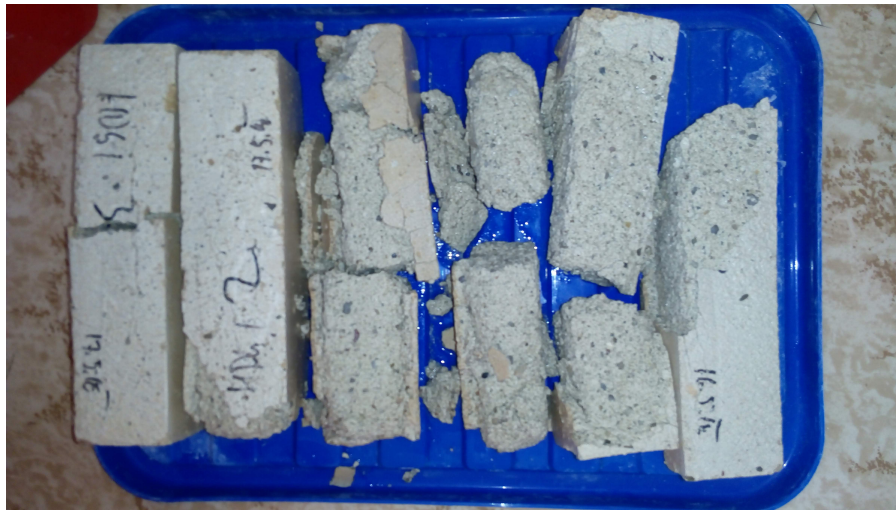
FIGURE 4. DG 1 and DG 5 (three of each from left to right) specimens after durability test.
