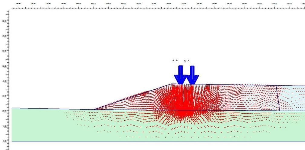
FIGURE 2. Total deformation caused by additional load from the belt stacker.
