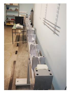
FIGURE 1. SHPB test apparatus at the University of Maribor.
