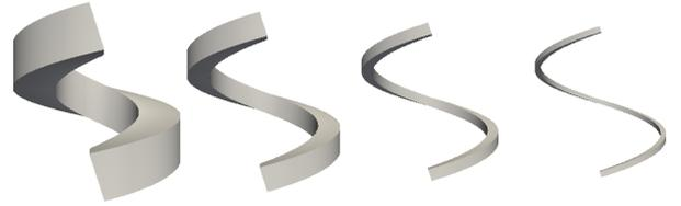
FIGURE 5. Helicoidal spring geometry for different thickness/length ratios: 0.1, 0.05, 0.025, 0.0125.
