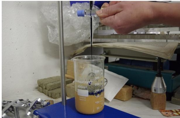
FIGURE 2. Methylene blue dye is dosed into earth sample.
