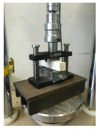
FIGURE 9. Three point flexural test technique [8].
