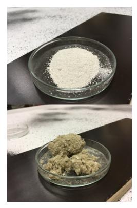
FIGURE 2. Fine milled gypsum and separated paper.
