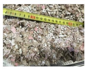
FIGURE 3. Crushed plaster boards with paper.
