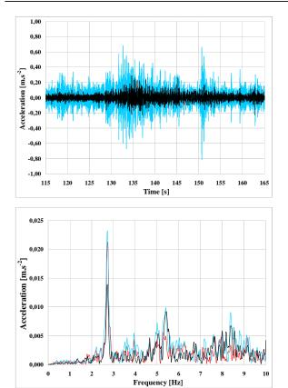
FIGURE 9. IBB, dynamic response of the stand – Bouncing – axes y [3].
