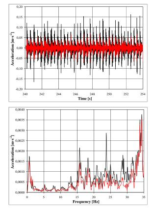
FIGURE 6. Ice-hockey, dynamic response of the stand - Hand-clapping [2].
