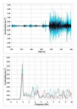
FIGURE 8. IBB, dynamic response of the stand – Hand-clapping after shoot [3].
