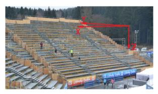
FIGURE 2. Location of sensors at the grandstands and measuring axis sensors [3].
