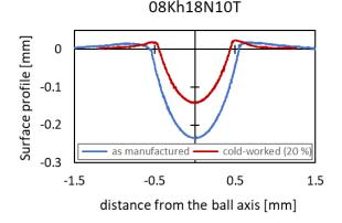
FIGURE 9. Cross-sectional profile of the spherical indent in undeformed a cold deformed 08Kh18N10T steel.
