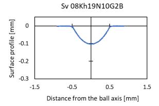
FIGURE 8. Cross-sectional profile of the spherical indent in Sv 08Kh19N10G2B steel.
