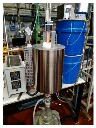
FIGURE 4. The apparatus for high-temperature oxidation.
