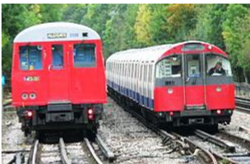
FIGURE 2. Cars for subsurface and deep-seated London Underground lines [3]
