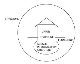
FIGURE 1. Interaction of structure and subsoil
