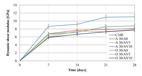
FIGURE 3. Development of dynamic shear modulus of the samples with slaked lime.
