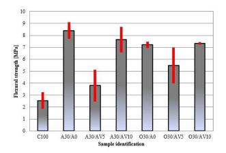
FIGURE 4. Flexural strength of the samples with slaked lime.
