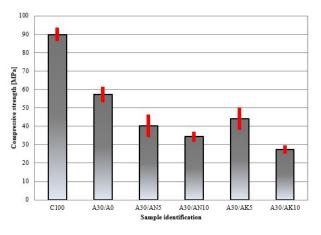
FIGURE 9. Compressive strength of the samples with water-glass.
