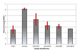
FIGURE 8. Flexural strength of the samples with water-glass.
