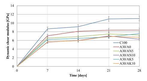
FIGURE 7. Development of dynamic shear modulus of the samples with water-glass.
