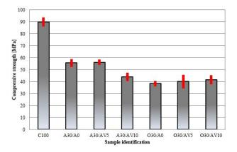
FIGURE 5. Compressive strength of the samples with slaked lime.
