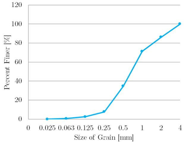
FIGURE 4. Grain curve of sand.
