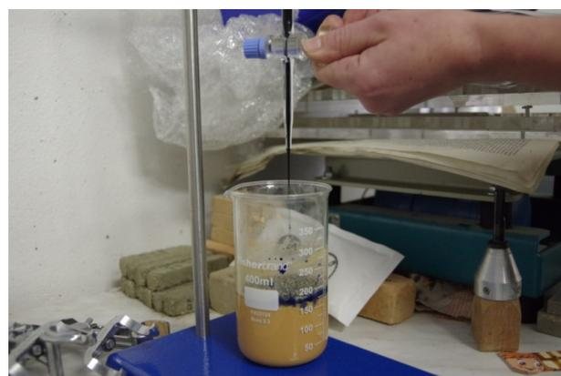
FIGURE 1. An earth sample with methylene blue solution.
