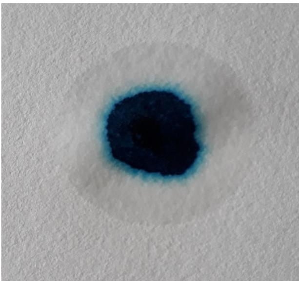
FIGURE 3. A result of methylene blue test.
