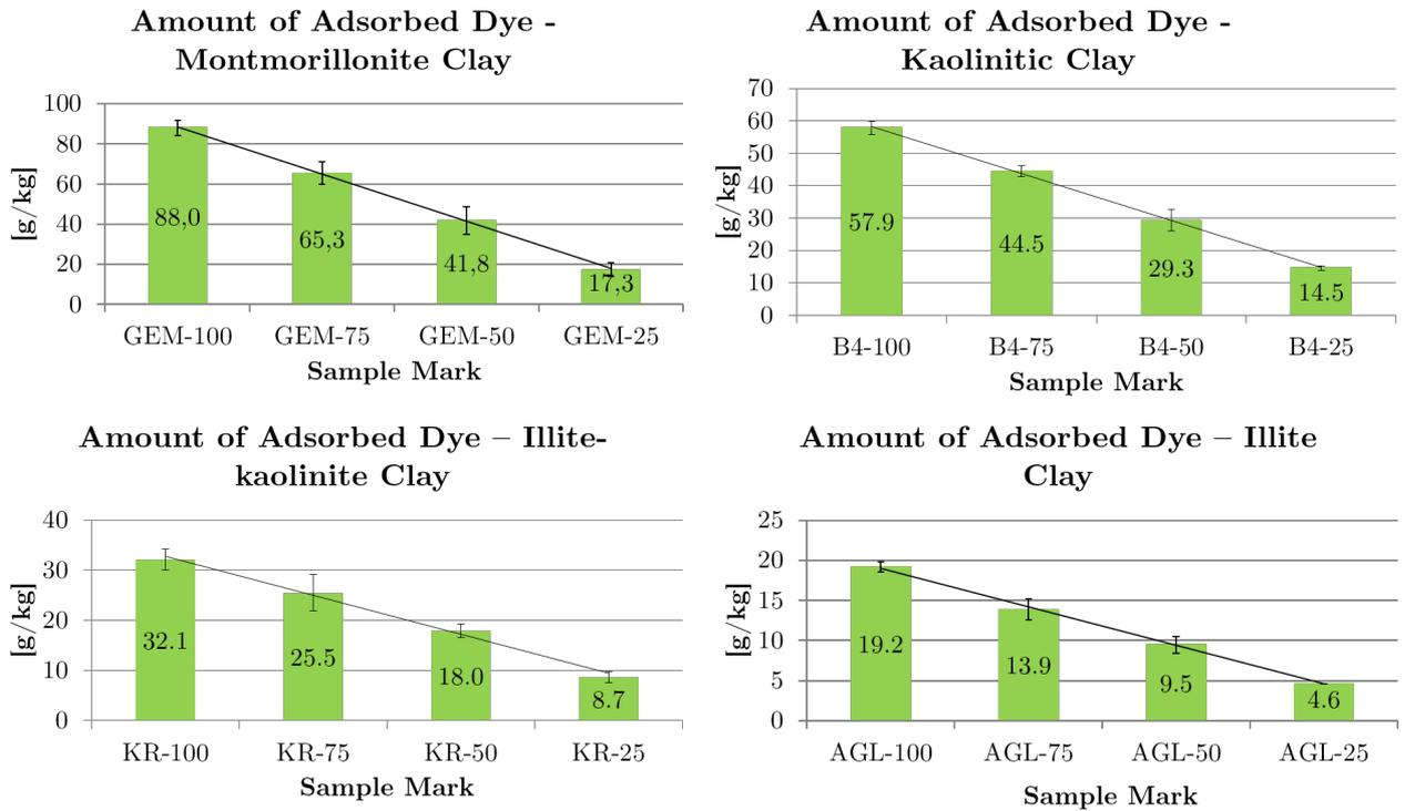
FIGURE 7. Amount of adsorbed methylene blue dye by clay.
