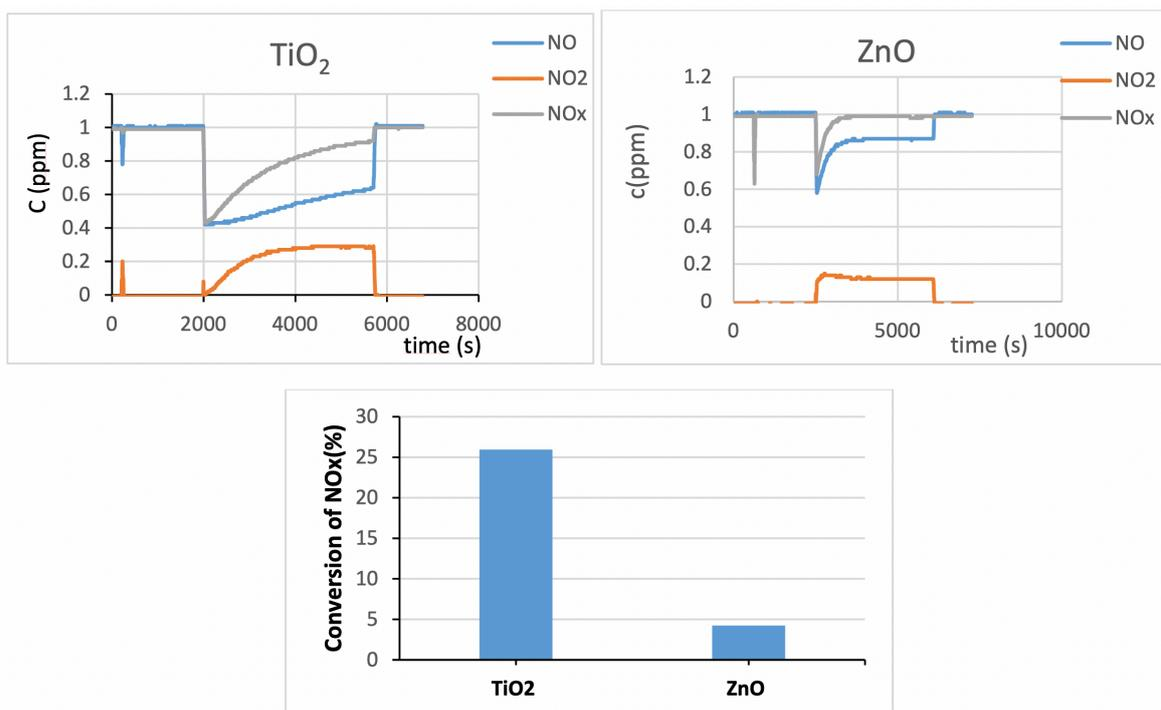
FIGURE 1. NO<sub>x</sub> abatements for TiO<sub>2</sub> and ZnO nanoparticles under UV irradiation.
