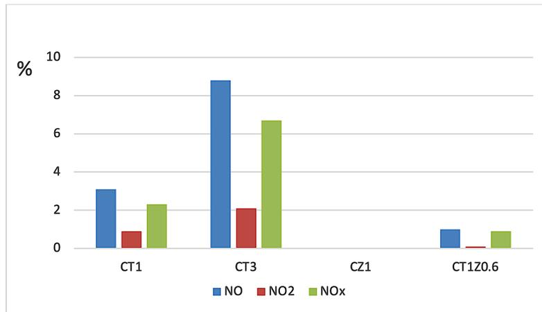
FIGURE 4. NO<sub>x</sub> removal under UV irradiation over CT1, CT3, CZ1 and CT1Z0.6.
