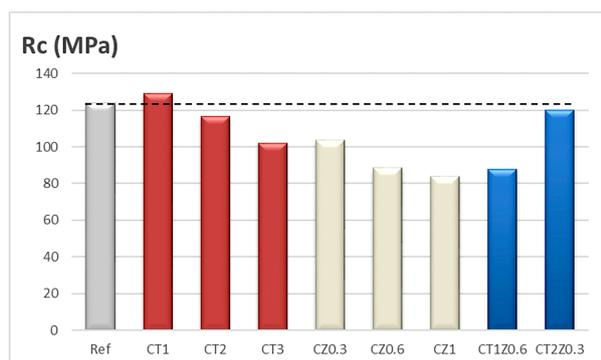
FIGURE 2. Compressive strength of HPC samples.
