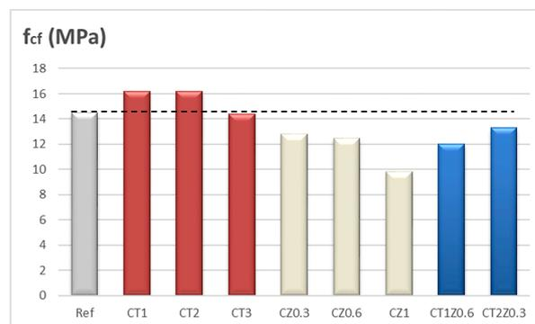
FIGURE 3. Flexural strength of HPC samples.
