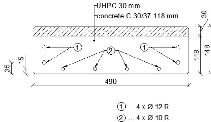
FIGURE 2. Typical geometry of the strengthened panels after the UHPC layer application [14].
