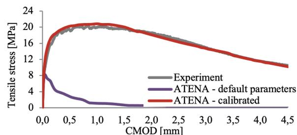
FIGURE 5. The experimental force-CMOD curve compared with the FE analysis results (with default material parameters and after the calibration procedure).
