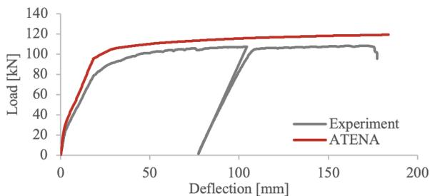
FIGURE 6. The experimental loading curve of strengthened panels compared with the ATENA simulation with material parameters based on the prior calibration procedures.
