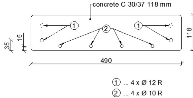
FIGURE 1. A typical geometry of the non-strengthened panels based on destructive investigations.
