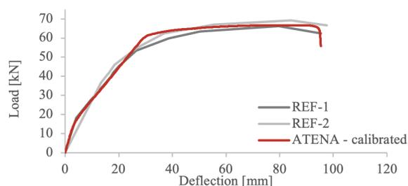
FIGURE 4. The experimental loading curves of the tested non-strengthened panels compared with the calibrated ATENA simulation.
