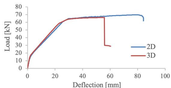
FIGURE 3. A comparison between the 2D and 3D loading curve - a reference panel with default material parameters.
