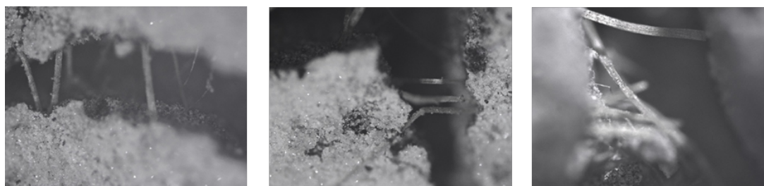
FIGURE 7. Optical microscographs image (x5) of lightweight cement blocks after compression test.
