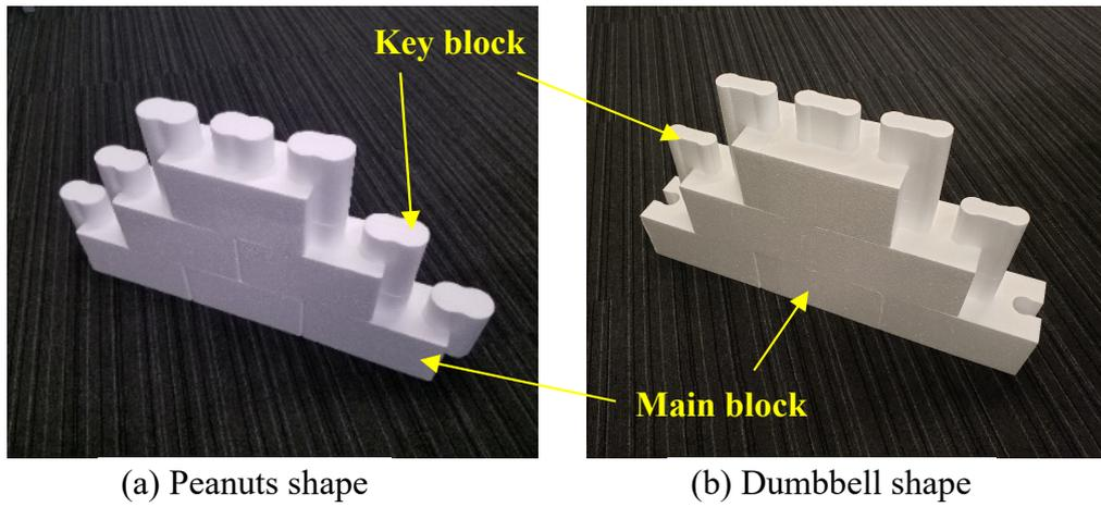
FIGURE 3. Construction of the proposed block walls.
