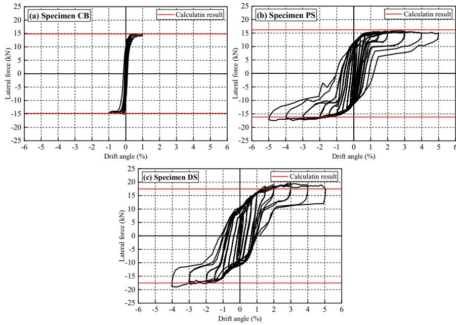
FIGURE 9. Lateral force-drift angle relationships of each specimen.
