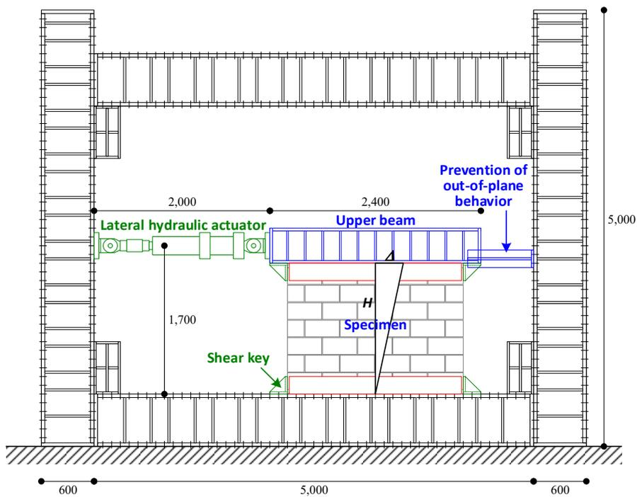
FIGURE 5. Loading system (unit: mm).
