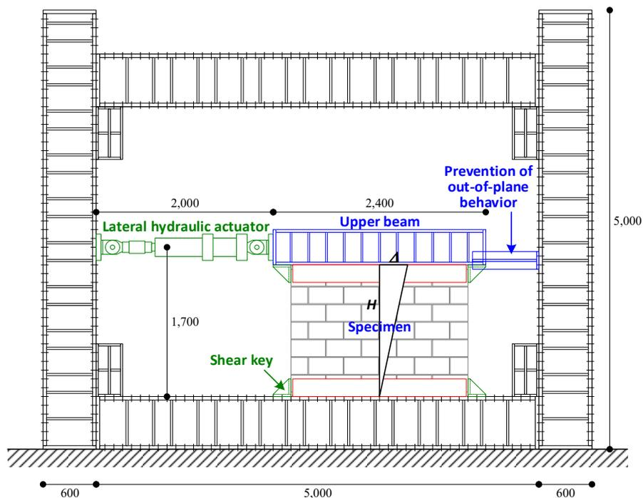
FIGURE 5. Loading system (unit: mm).
