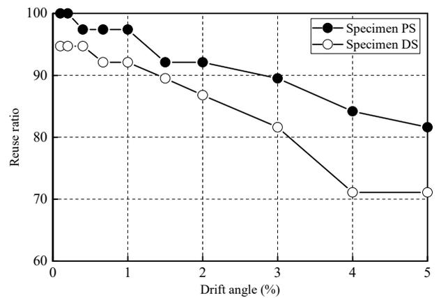
FIGURE 13. Reuse ratios of the main blocks of Specimens PS and DS.
