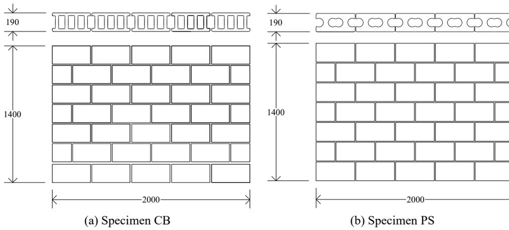
FIGURE 4. Details of typical and proposed concrete block wall specimens (unit: mm).
