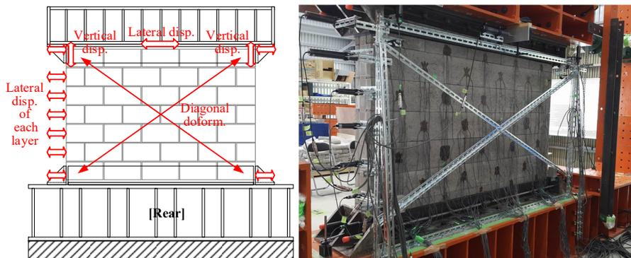
FIGURE 7. Measurement system.
