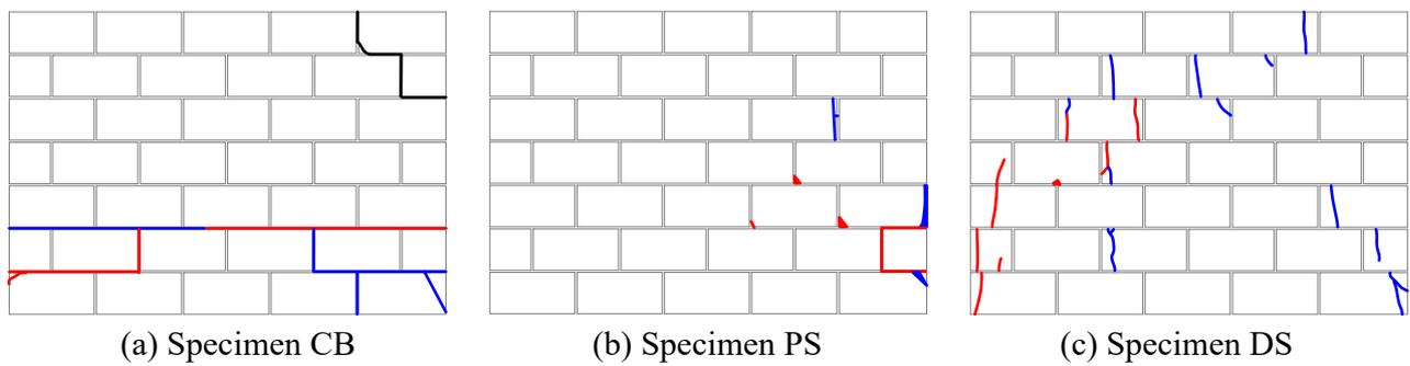
FIGURE 8. Final crack patterns (Blue: Positive dir., Red: Negative dir., Black: Initial cracks).
