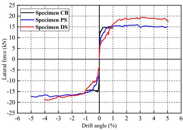
FIGURE 10. Skeleton curves of each specimen.
