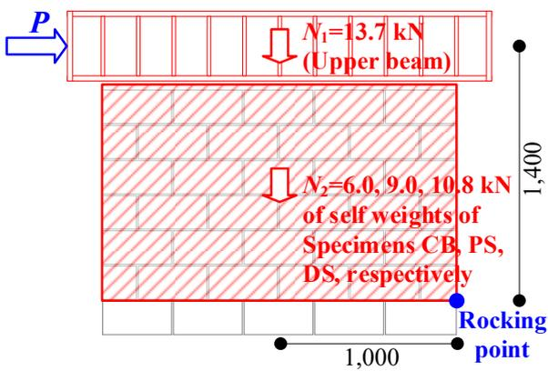
FIGURE 11. Lateral load  $P$  due to rocking mechanism.
