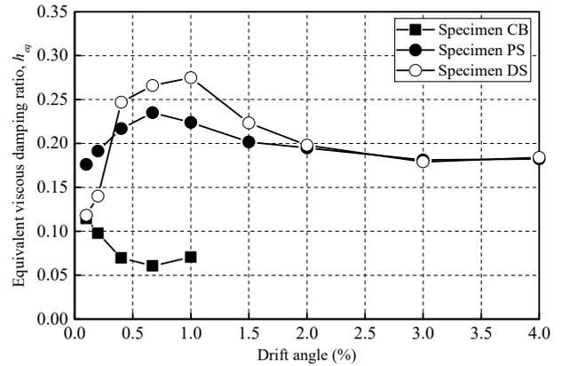
FIGURE 12. Equivalent viscous damping ratios.
