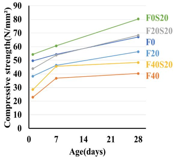
FIGURE 2. Compressive strength of mortar under 20 °C-sealed curing.
