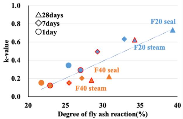
FIGURE 7. Relationship between k-value and degree of fly ash reaction.
