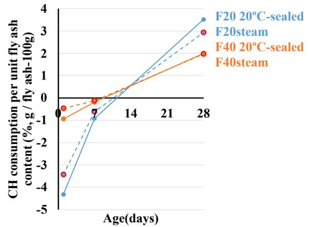
FIGURE 5. CH consumption per unit fly ash content with age.
