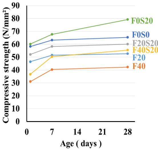
FIGURE 1. Compressive strength of mortar under steam curing.
