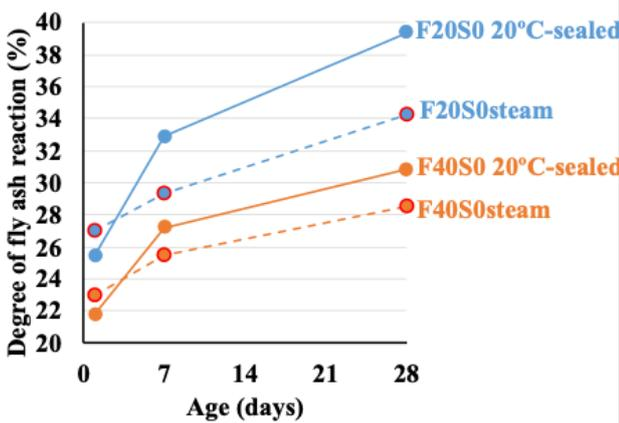
FIGURE 6. Degree of fly ash reaction with age.
