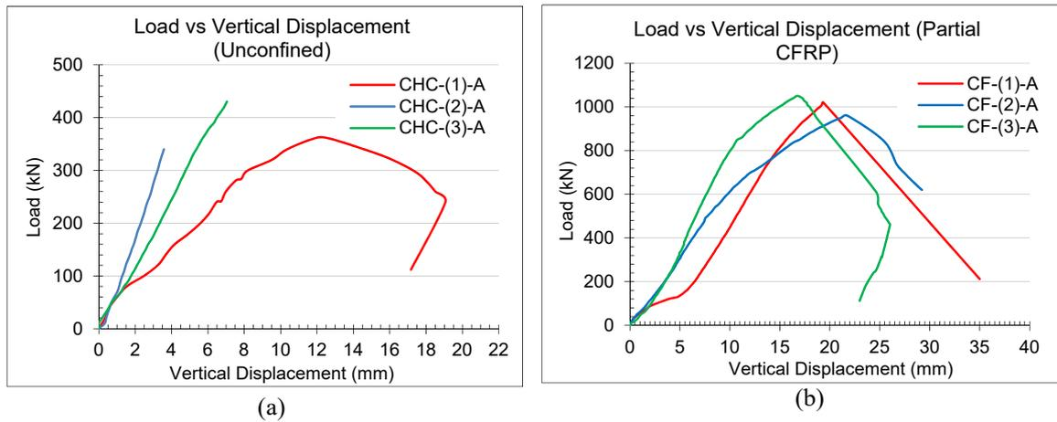
FIGURE 4. Load vs Vertical Displacement; (a) Unconfined CHRCC (b) Partial CFRP CHRCC.
