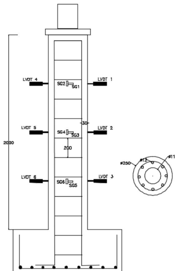
FIGURE 1. Detail of Specimen (dimensions in mm).
