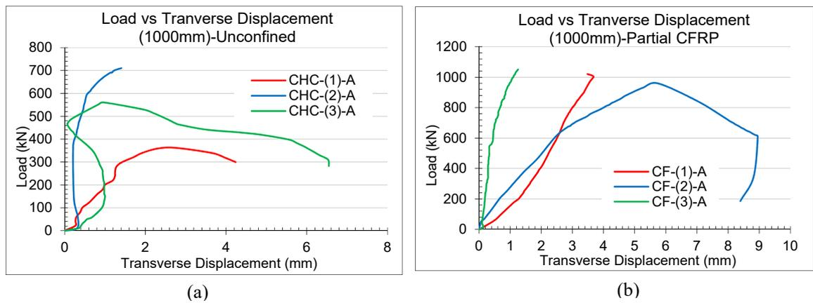
FIGURE 5. Load vs Transverse Displacement; (a) Unconfined CHRCC (b) Partial CFRP CHRCC.
