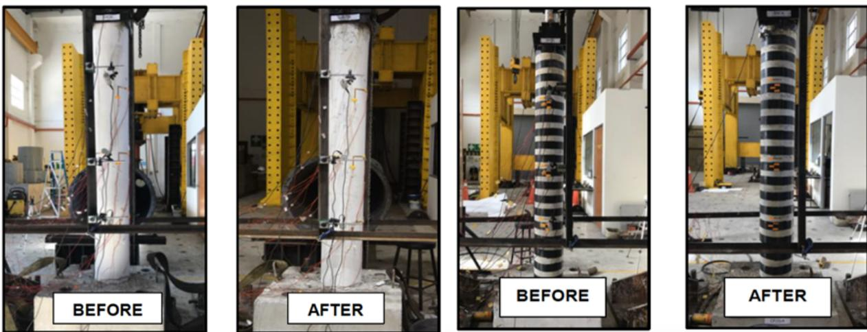
FIGURE 3. Failure behaviour of CHRCC Before and After Concentric Loading.
