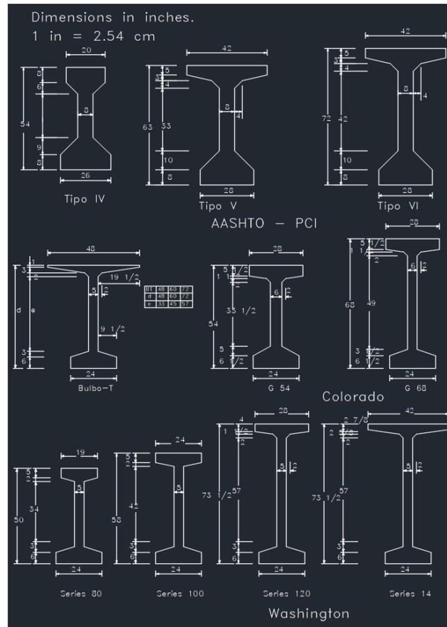
FIGURE 2. Modified girder analyzed (AASHTO, Bulb T, Colorado and Washington).
