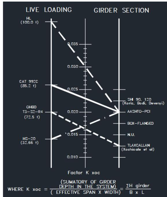
FIGURE 4. Graphic definition of  $K_{xoc}$ , according to live loading and girder type.
