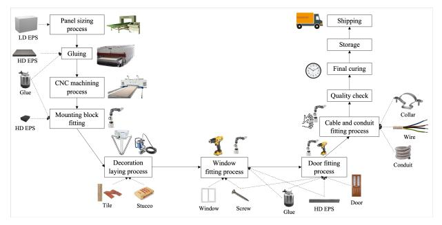
FIGURE 4. Smart Construction Factory production process and used machinery.
