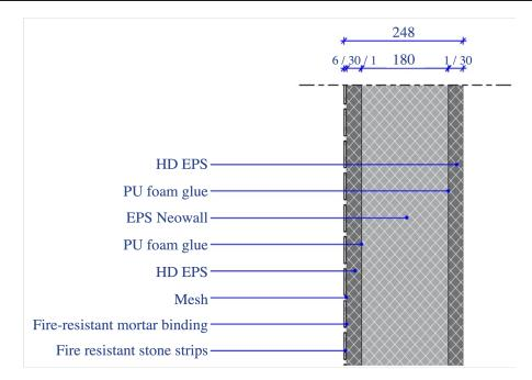
FIGURE 1. Assembly of the wall component design: sandwich panel.
