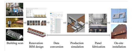
FIGURE 3. Future INDU-ZERO construction supply chain process overview.
