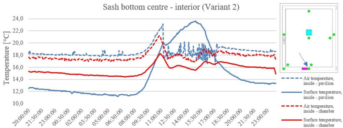
FIGURE 6. Temperature courses for the bottom of windows sash. Difference of about 3°C in surface temperatures.
