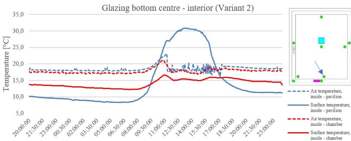
FIGURE 5. Temperatures courses for the bottom of glazing. Variant 2 with non-steady indoor temperature. Difference of about 4°C in surface temperatures.
