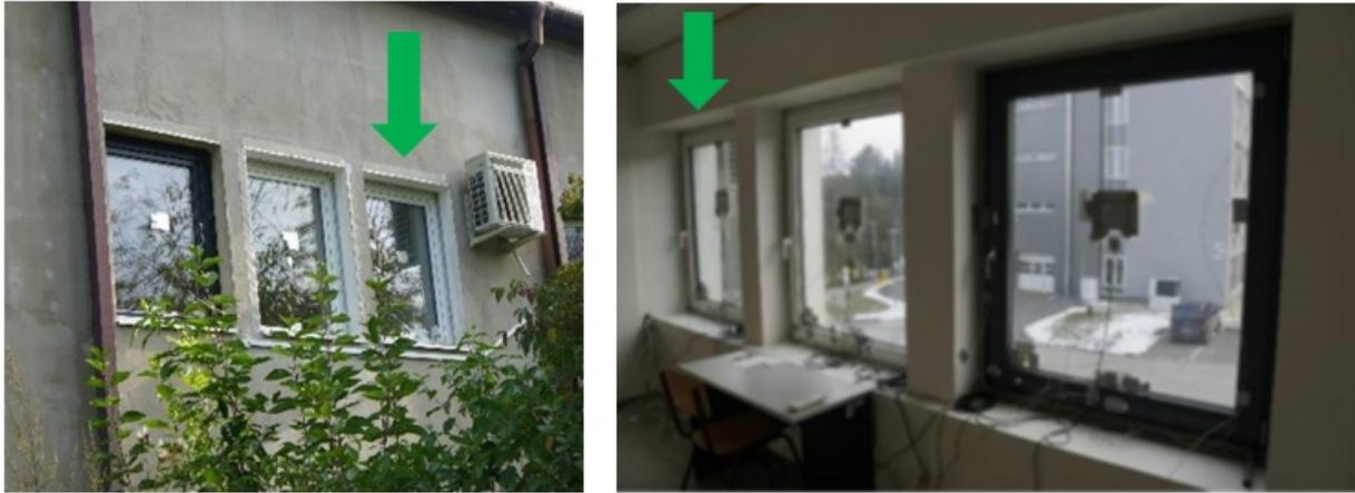
FIGURE 1. External and internal view of the built-in plastic window in the test laboratory.
