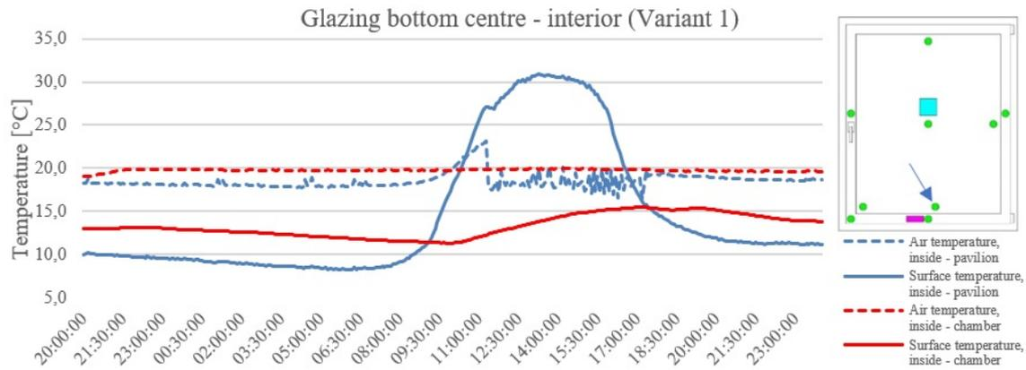
FIGURE 4. Temperature courses for the bottom of glazing. Variant 1 with constant indoor temperature. Difference of about 3°C in surface temperatures.
