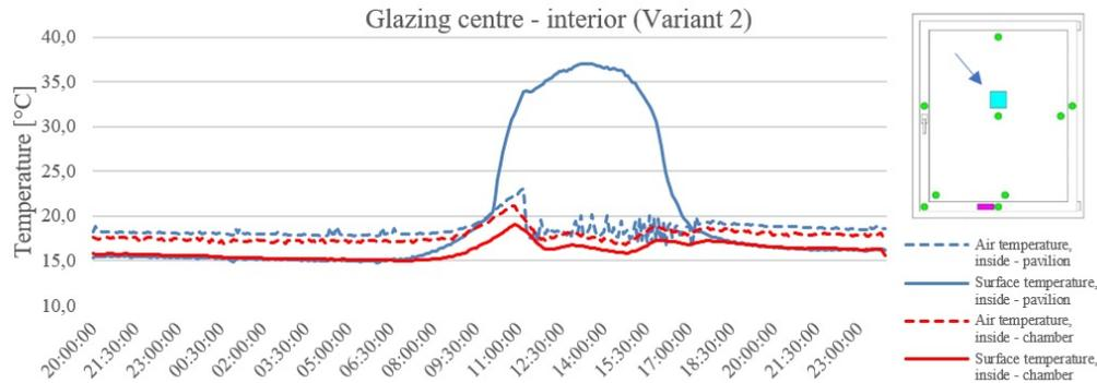
FIGURE 3. Temperature courses for the Centre of glazing. Very good match of courses at the night (without solar radiation).
