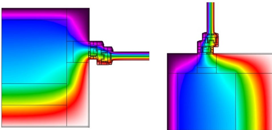
FIGURE 7. Temperature waveforms according to the Therm software simulation at the lining and sill location.
