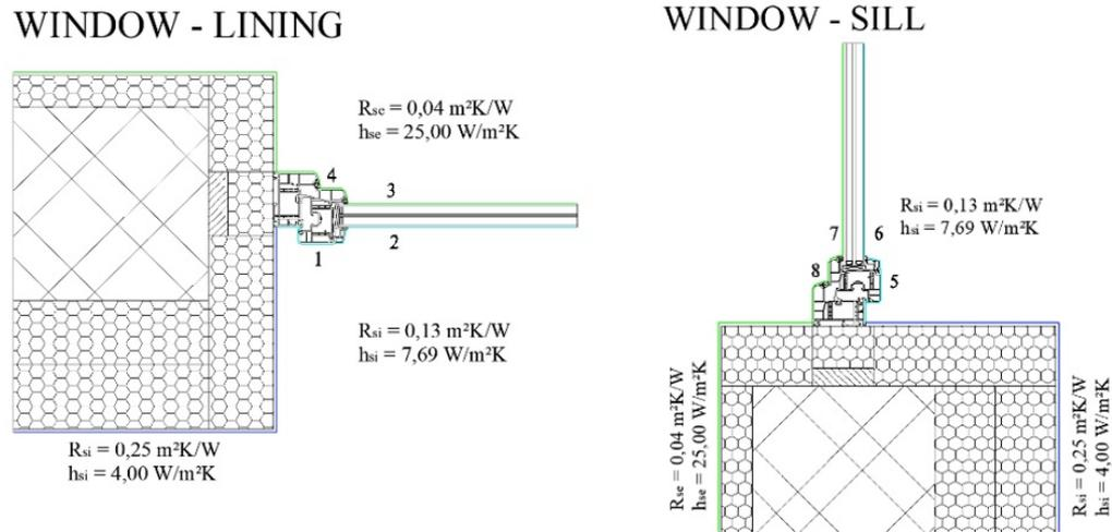
FIGURE 2. Detail of the window in the wall of the laboratory. Marked positions for comparison of surface temperatures.
