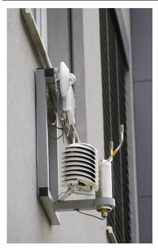
FIGURE 8. FMS with the new type of shield on the facade.
