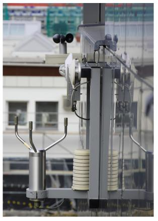
FIGURE 6. FMS with the previous type of shield on the facade.
