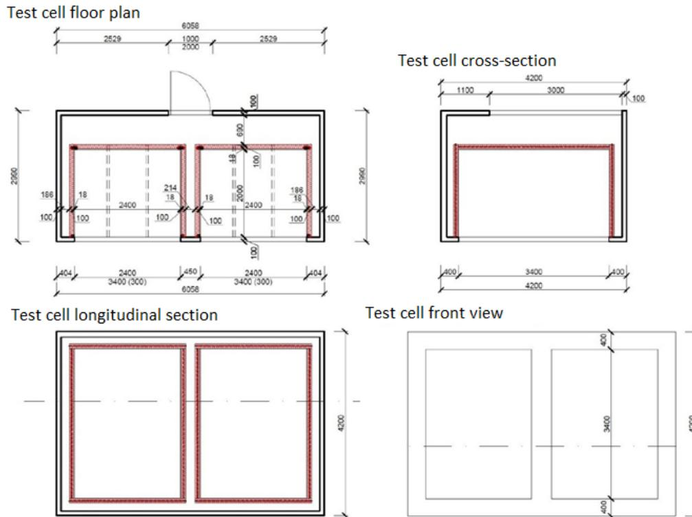
FIGURE 1. Construction schemes of an experimental test cells Twin Rooms for testing advanced facade elements in real conditions of outdoor climate.
