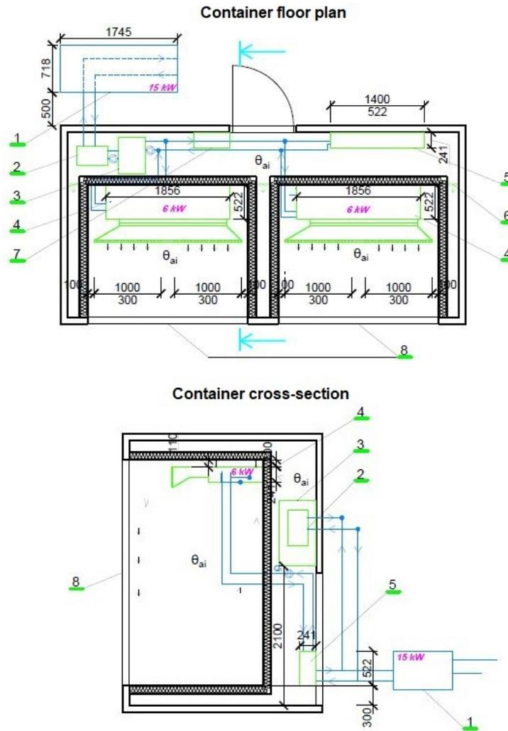
FIGURE 2. Construction scheme of technological equipment of an experimental test cells Twin Rooms. 1 – Cooling source,  $Q_c = 16.4\text{ kW}$ , MEX EA 117 Z C, 2 – Plate heat exchanger – part of the supply of the cooling source, 3 – Water tank – storage tank Galmet 140 l, 4 – Pipe fancoil NXKT3-V1000, 5 – Sill fancoil NXKH3-V600, 6 – Circulating fans – homogeneous thermal field, 7 – Electrical switchgear, 8 – Opening for mounting a new facade sample.
