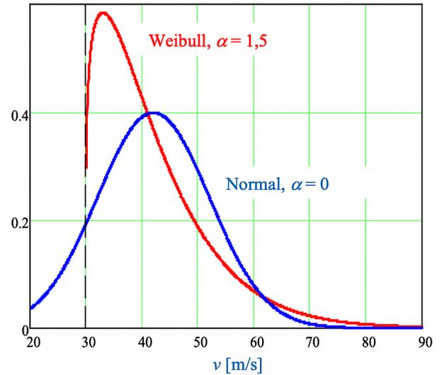
FIGURE 1. Weibull and normal distribution for  $\mu = 42$  m/s and  $\sigma = 10$  m/s.
