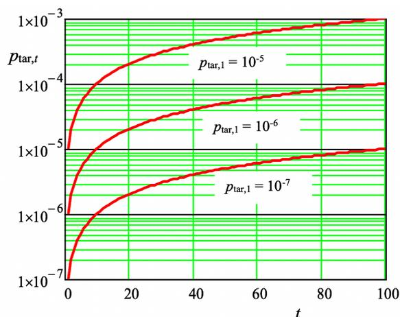
FIGURE 3. Variation of the target probabilities  $p_{\text{tar},t}$  with reference time  $t$  in years for basic probabilities for one year -  $p_{\text{tar},1} = 10^{-5}$ ,  $10^{-6}$  and  $10^{-7}$ .
