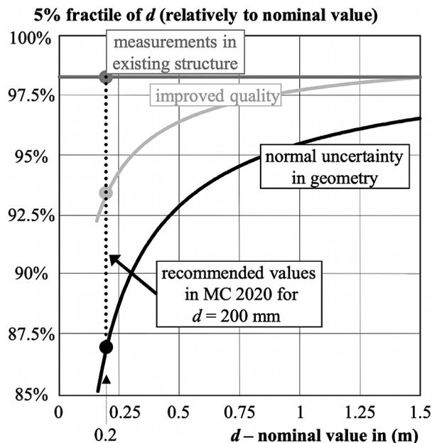
FIGURE 2. Effective depth - 5% fractiles as a function of nominal value.
