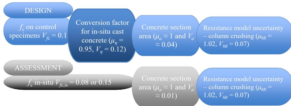
FIGURE 1. Basic variables considered in resistance model for short columns in design and assessment situations.
