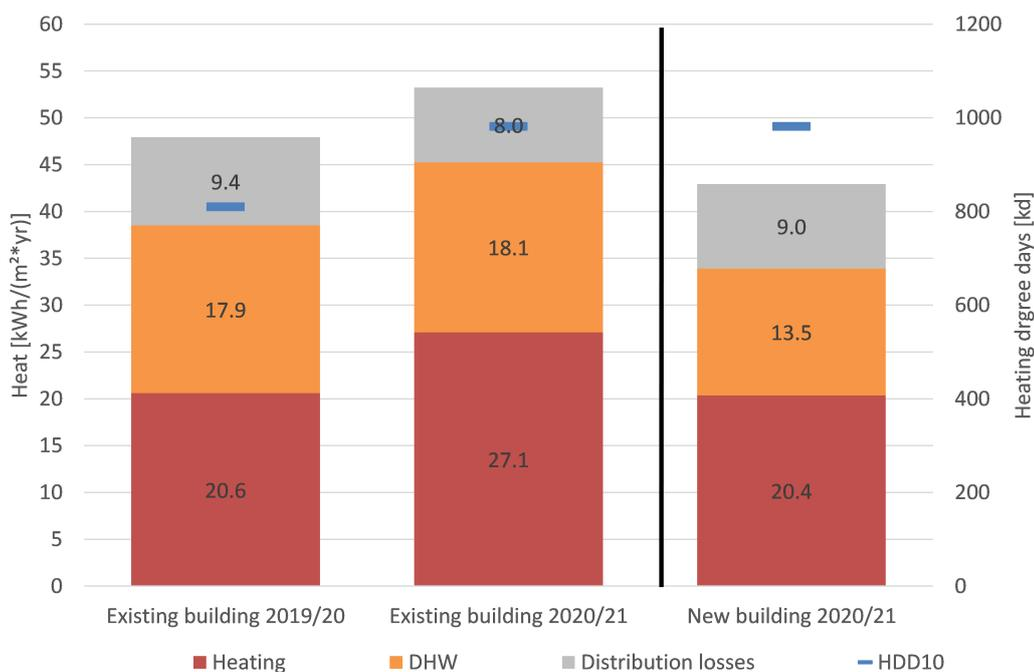
FIGURE 4. Heat consumption for heating, DHW and distribution losses of the refurbished (left and middle column, two heating periods) and the new building (right column, one heating period) as well as heating degree days on site.
