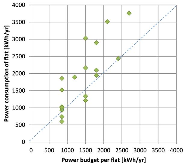
FIGURE 6. Power consumption per flat over power budget per flat for the new building 2020/21.
