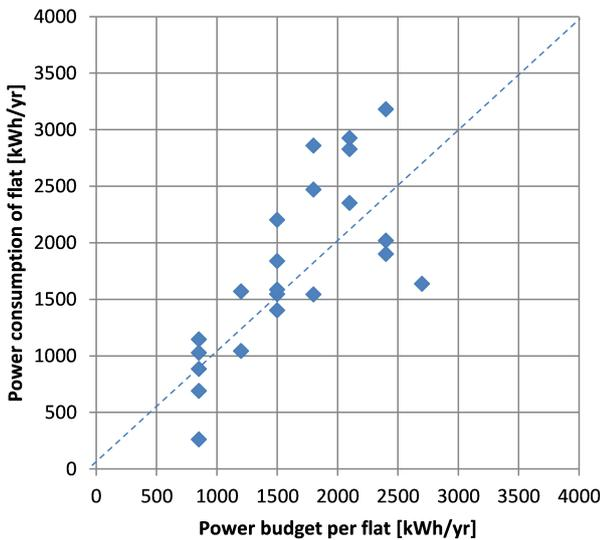
FIGURE 5. Power consumption per flat over power budget per flat for the refurbished building 2020/21.
