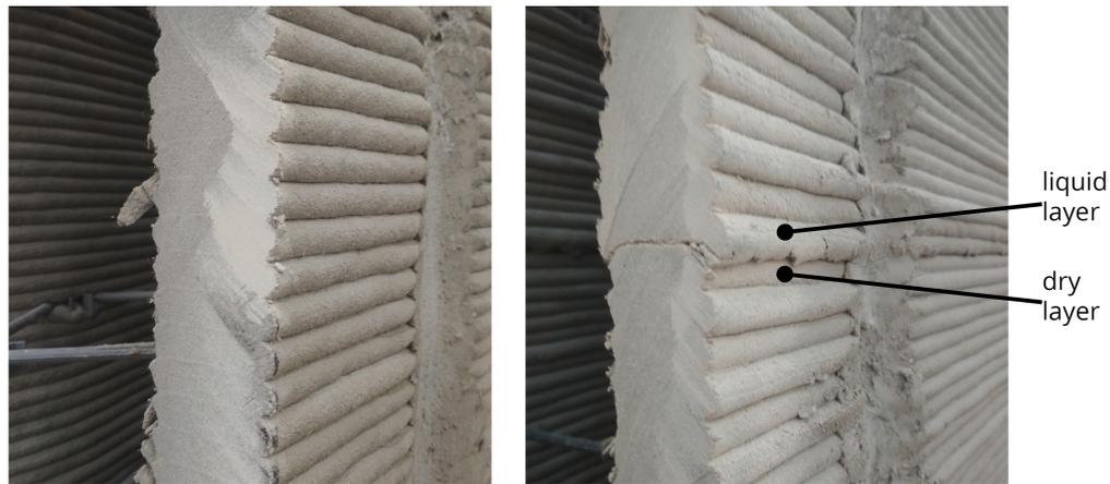
FIGURE 5. Optimal consistent material (left) and inconsistent material (right).
