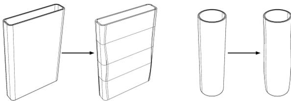
FIGURE 3. The principle of buckling.
