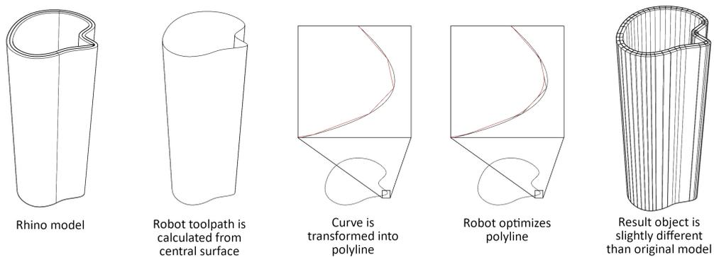
FIGURE 2. Robot optimization of the path.
