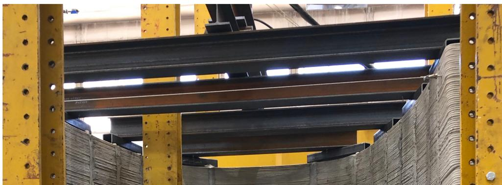
FIGURE 8. Load distribution system.
