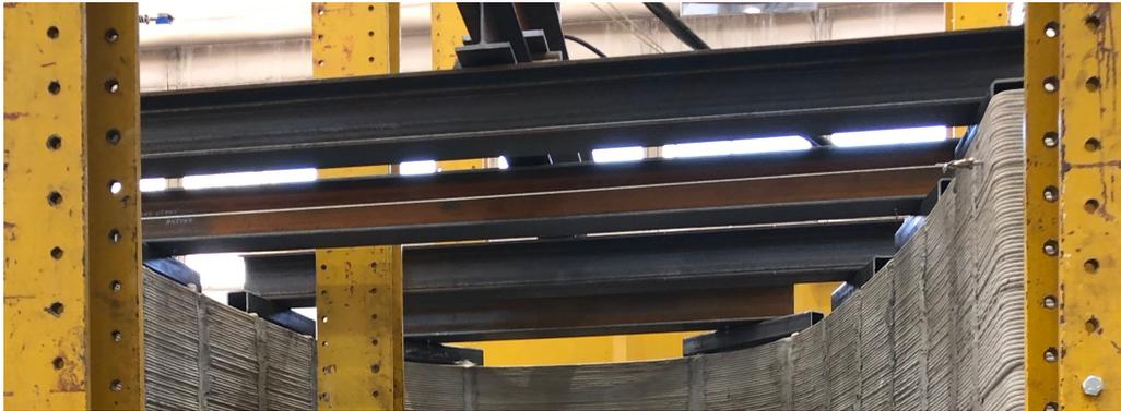
FIGURE 8. Load distribution system.
