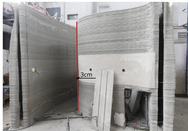
FIGURE 4. Buckling of the 3 meter high wall.
