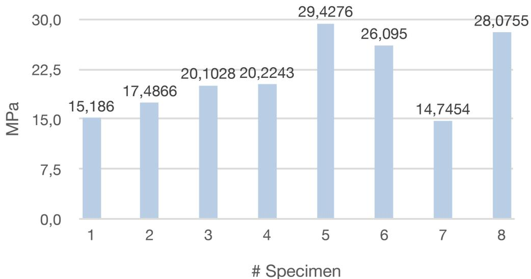
FIGURE 13. The compressive strength of experimentally investigated specimen.
