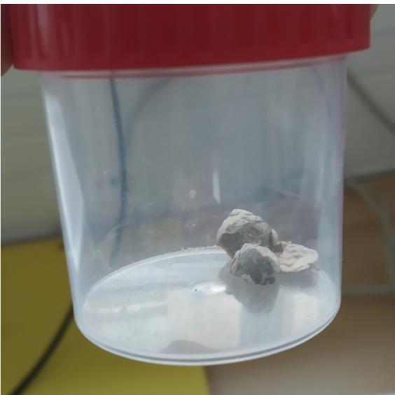
FIGURE 2. Sample of recycled concrete after the MICP process.
