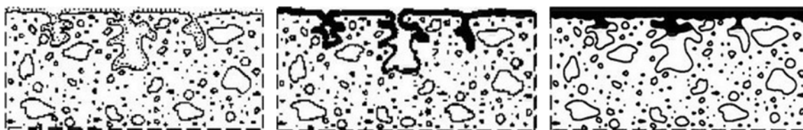
FIGURE 1. Hydrophobic impregnation, impregnation, coating (from the left side) [2].
