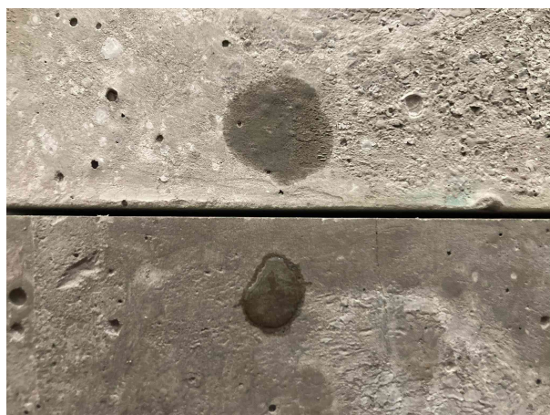
FIGURE 3. The influence of impregnation on the size of the wetting angle.
