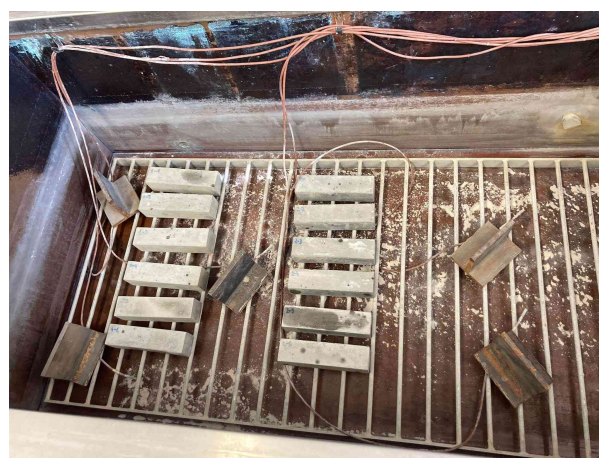
FIGURE 8. Test specimens placed in a freezer box.
