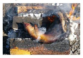
**Figure 10:** Specimen 1. Specimen temperature: 379°C. Fire temperature: >900°C. Time: T+23. Efford 2016.
