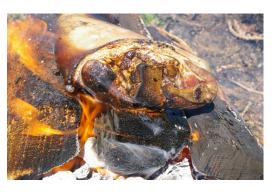
**Figure 8:** Specimen 1. Specimen temperature read 491°C. Fire temperature read >900°C. Time: T+14. Efford 2016.
