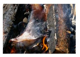
**Figure 12:** Specimen 2. Specimen temperature: 480.2°C. Fire temperature: >900°C. Time: T+24. Efford 2016.
