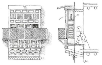
Figure 3. Details of Mashrabiya in elevation and section view (Ragette 2006)
