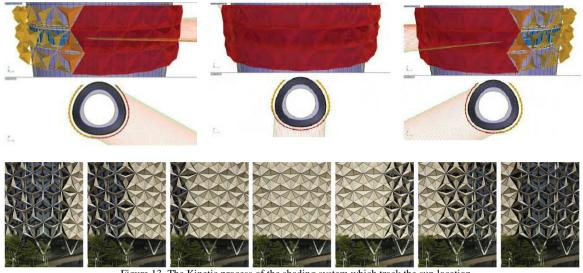
Figure 13. The Kinetic process of the shading system which track the sun location
