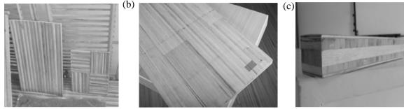
Figure 5. (a) Samples cut out from DPLM board , (b) DPLM board after treated (c) DPLM double board as a sandwich panel.
