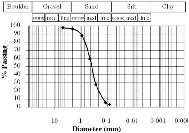
Figure 16. The sieve analysis of specimen 10 at 89 E km at Sarapum
