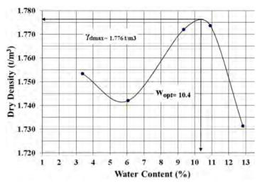
Figure 21. Modified proctor test for specimens from 88.1E km to 89E km at Serapum area
