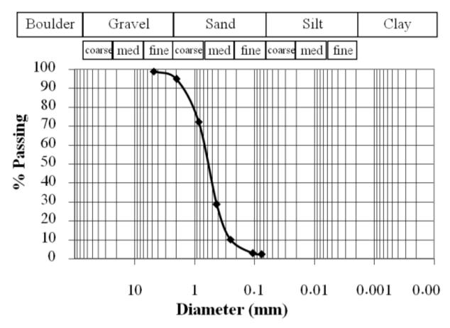
Figure 15. The sieve analysis of specimen 9 at 88.5E km at Sarapum
