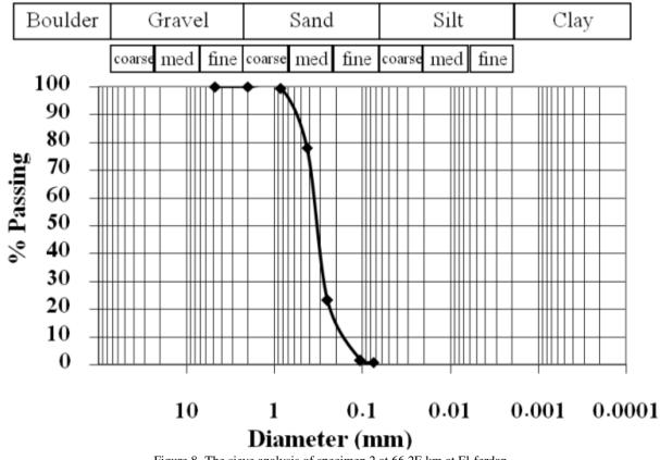
Figure 8. The sieve analysis of specimen 2 at 66.2E km at El-ferdan
