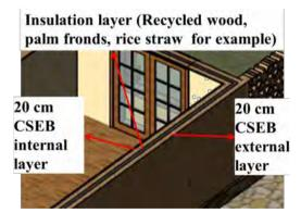
Figure 3. Isometric of the multi-shell wall for the energy efficient envelope of the residential building.
