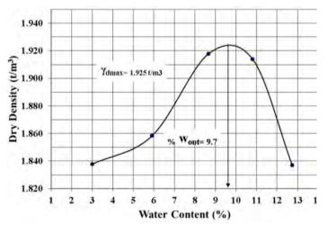
Figure 20. Modified proctor test for specimens from 67.3E km to 69.1E km at Elferdan area
