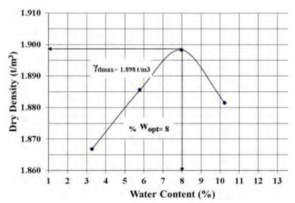
Figure 22. Modified proctor test for specimens from 89E km to 90.5E km at Serapum area
