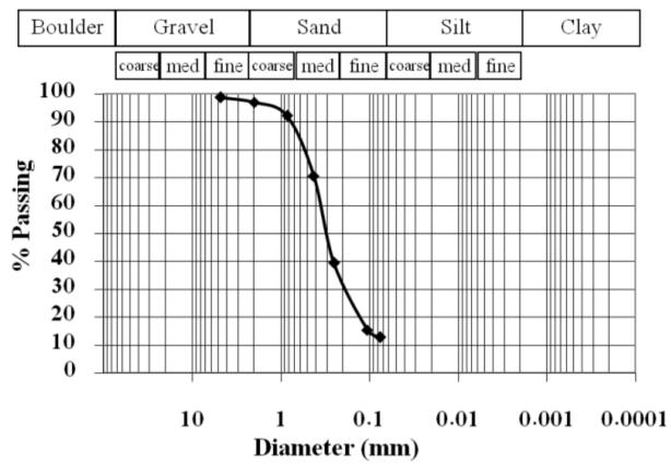
Figure 13. The sieve analysis of specimen 7 at 69.1E km at El- ferdan
