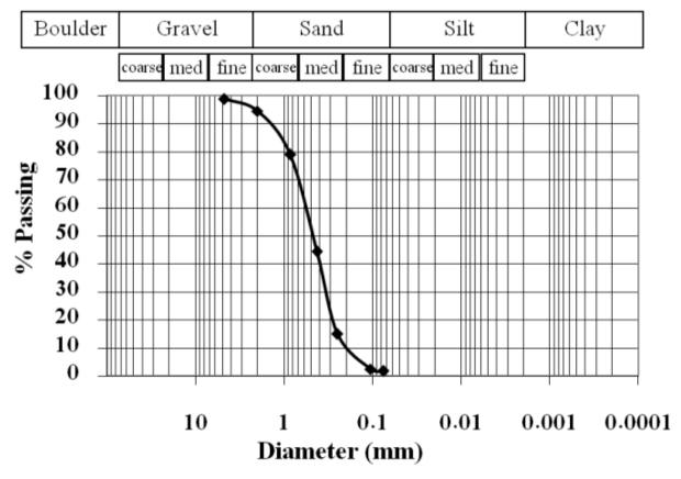
Figure 10. The sieve analysis of specimen 4 at 67.3E km at El-ferdan
