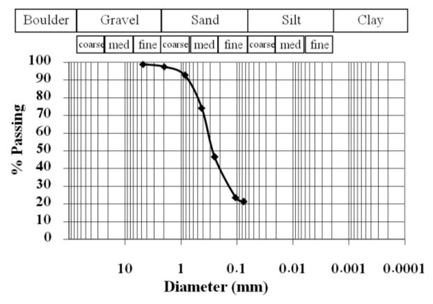
Figure 12. The sieve analysis of specimen 6 at 68.5E km at El-ferdan
