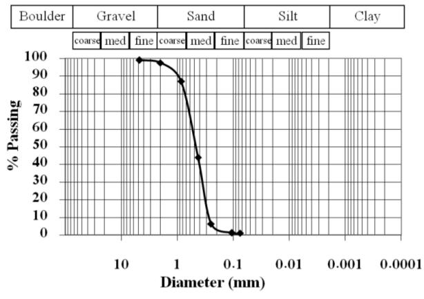
Figure 11. The sieve analysis of specimen 5 at 67.9E km at El-ferdan
