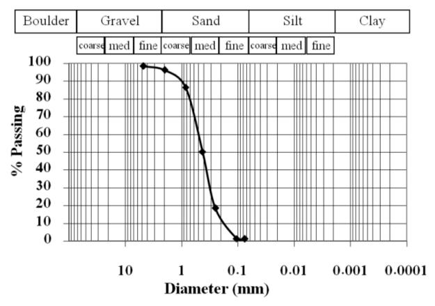
Figure 14. The sieve analysis of specimen 8 at 88.1E km at Sarapum
