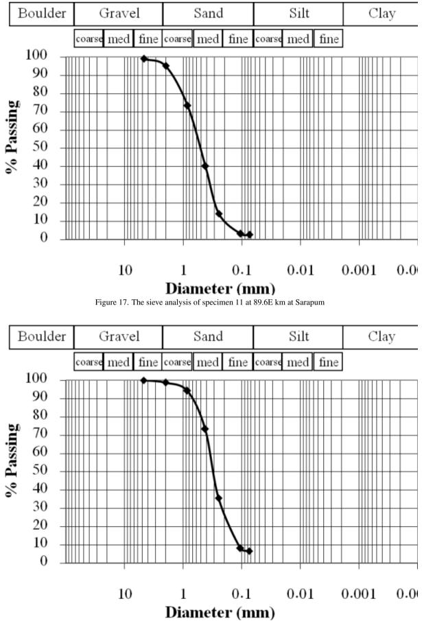
Figure 18. The sieve analysis of specimen 12 at 90.5E km at Sarapum
