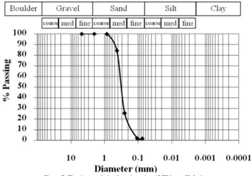
Figure 7. The sieve analysis of specimen 1 at 65.7E km at El-ferdan
