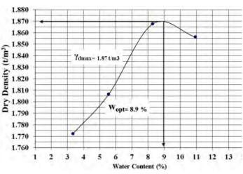
Figure 19. Modified proctor test for specimens from 65.7E km to 67.3E km at Elferdan area
