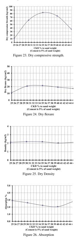
Q = -0.5891r2 + 42.49r - 682.71Where Q = Dry compressive strength at 28 days(k/cm2) (3) r = CKD ratio to sand weight (%)
