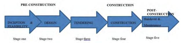
Figure 2. Construction Project Management. Stages (K.S., I. H. S. (2002).
