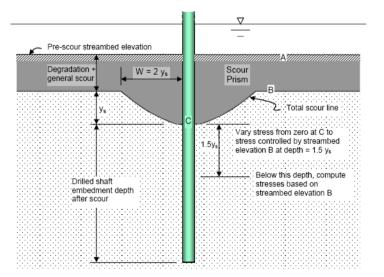
Figure 2. The effect of scour on bridge foundations (AASHTO LRFD Bridge DesignSpecifications, 2007).
