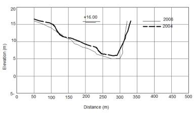
Figure 15. Cross section No.2 at years 2004 and 2008
