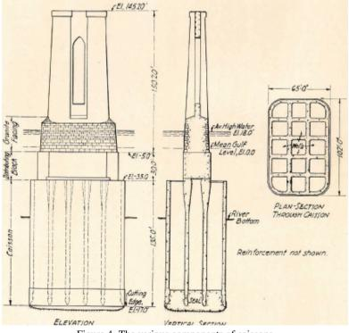
Figure 4. The various components of caissons
