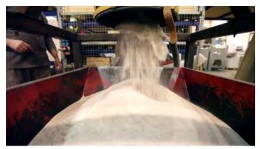
Figure 13. TheExcessive sands while printing process
