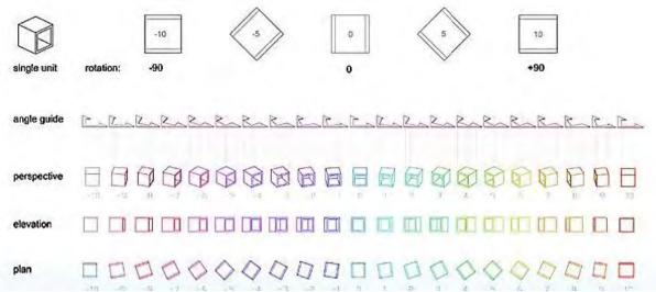
Figure 6. SilkWall. The angles of rotation of the cement blocks were constrained to 21values. Wooden formats were given by the architect to educate the manufacturershow to distribute the pieces to the right position.
