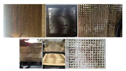
Figure 16. Palm leaves mat before and after laser cut and how it helped to change the users perception to the material.
