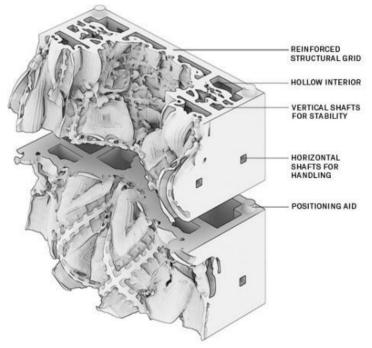
Figure 9. Isometricassembly detail of the mass
