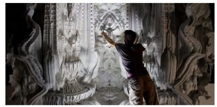
Figure 14. The Intricate Grotesque after finishing and it shows a new phase in additive manufacture and its impact on architecture leading to generate classic forms though the processing phase was computationally done
