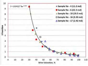
Figure 13. Leverett J-Functionfor the Upper Bahariya reservoir core samples
