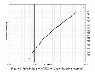
The Log-Log plot of RQI versus  $\emptyset_z$ , FZI histogram analysis and the cumulative probability plots allow picking out at least 9 HFUs and estimate FZI boundaries for these rock types. Table (1), summarizes all of these HFUs. Also, the value of intercept HFUs lines at  $\emptyset z$  equal one is mean FZI and will be used to calculate permeability.
