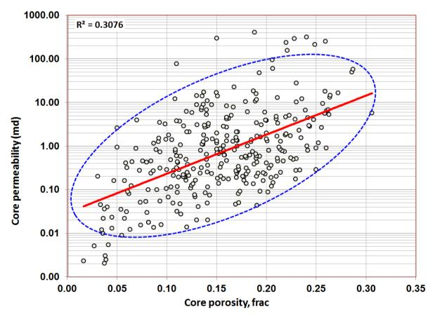
Figure 5. Core porosity versus core permeability for Upper Bahariya reservoir.
